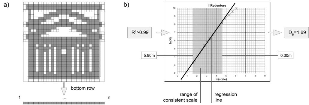
double-logarithmic graph with the number of boxes  $N_i$  versus scaling factor  $s_i$ , the slope of the regression line defines the box-counting dimension  $D_B$  (Figure 1b) for a certain range of scales (Foroutan-pour et al. 1999).
