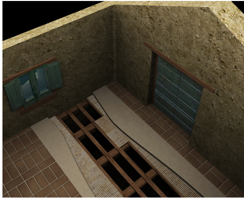
Figure 2 (Left) - the constructive system of the floor (internal view of the room on the first floor); (right) - rendered view of the constructive system of the pitch roof.
