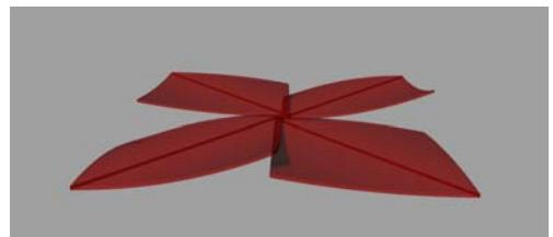
Thanks to the Hoadley's (1980) demonstration, that the wood from the centre of tree trunk warps more than the wood from its border, the system Ray 2 (figure 5) was developed. This fact enabled the overlapping on the diagonals' crossing, by its layering (figure 6).
