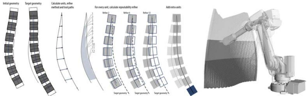
robotic machine assembles and adjusts acrylic structural units (dimensions 4cm x 4cm x 1 cm) within the overall structure and these are influenced by external changes that have occurred in the physical environment.
