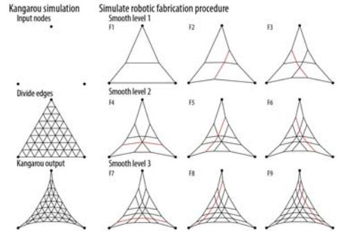
The process of smoothness is characterised as continually additive, where the designer is able to add new points to define the overall mesh system. Through the camera sensor, these points can be taken into account and used in other triangulated mesh systems. The new triangulations effect the existing system, triggering a new smoothness procedure that is continuously repeated until the required smoothness is achieved (Figure 7).
