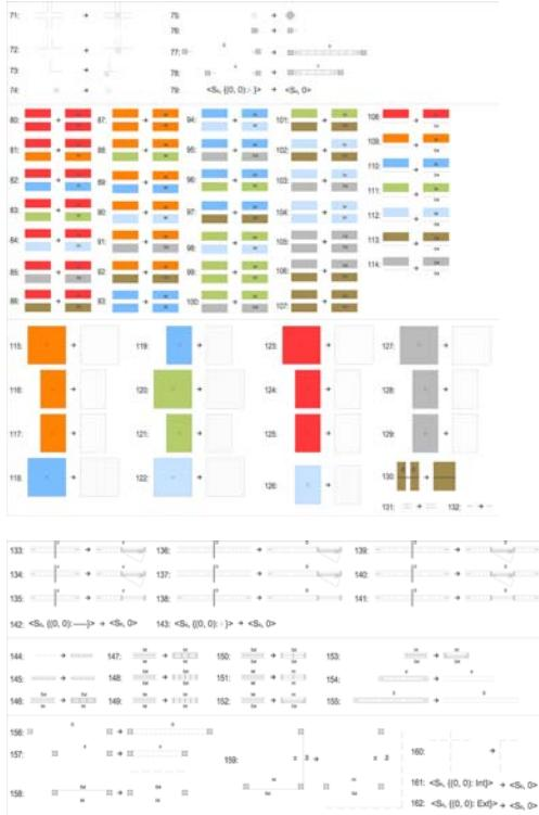
To aid the placement of wall panels in upcoming stages, rules 80 to 114 place a label *Ext* and *Int* indicating which side of each module is exterior and which is interior. These labels remain in the design for later use. The rule schemata 115 to 129 associate a floor panel for each space. Because each functional area is shaded with a different color the rules asso-
