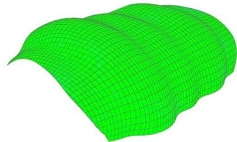
The first direction is created by a stream of parallel lines with a given distance among them. The second direction is created by a polar array of lines with a given angle of 5 degree among them. The intersec-
