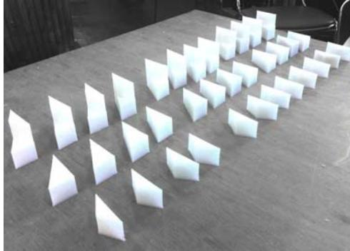
By combining these two manufacturing techniques, we can decrease the 3D-milling process. Only you have to do is ADD three-dimensional shapes (Figure 6). In addition, if we use the 3D-printed parts as a mould, the efficiency of the process should improve even further.
