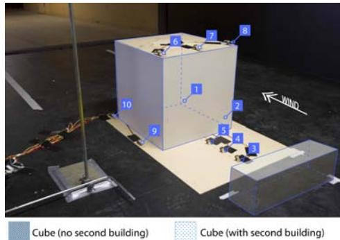
The experiment to test the sensor platform was designed to simulate of the canyon effect, an accelerated vortex of wind in the space between both a high building and lower building. The phenomenon is produced by a downward wind flow deflected by the high building facade to the ground level. The wind
