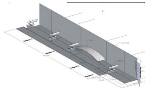
Above each screen, there is a curved surface of 2m height. This surface is a deflector that creates a wake region and low pressure layer at the top of the protec-
