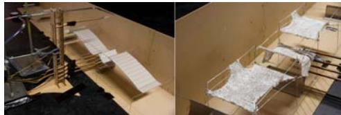
The most interesting observation of this visualisation was the fact that a roof with continuous surface produces an acceleration of wind speed in the region below. In contrast, if the roof is split in three parts
