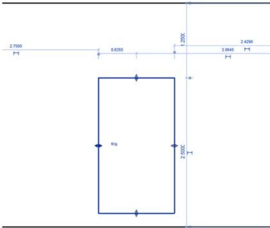
ric features a singular component will automatically adjust for every different sized or different shaped opening or wall (figure 2), automatically adapting other components to it such as floors.
