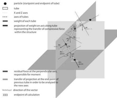
As moving from joint to joint apart from the compressive force that was generated from the weight of the current branch, the previous calculated force vector was also resolved into its new components. The perpendicular to the axis of the branch force compo-
