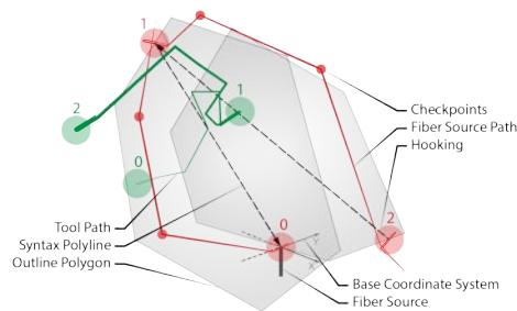
Figure 7 Based on the syntax polyline (black) is generated path of the fiber source (red), that is further translated into the end effector path (green).
