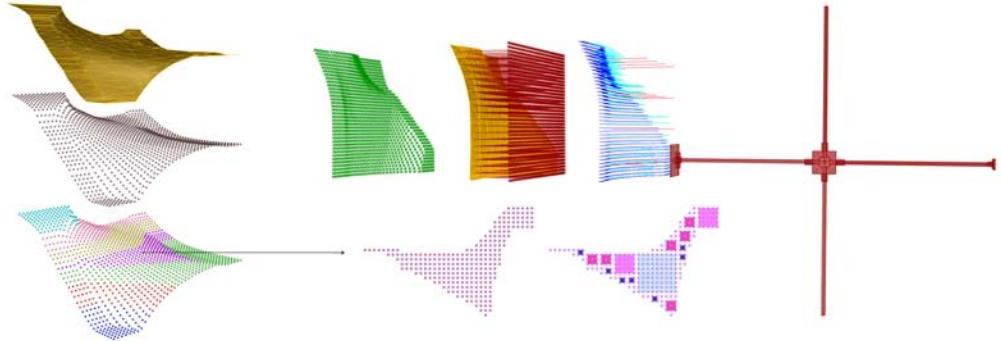
The K-Means algorithm partitioned the 1600 surface points into a set range of clusters (min 5, max 10) and return the solution with the smallest overall distance the robot had to travel to reach each cluster's mean (center point) and back. This allowed the calibration of each cluster separately, reducing substantially the path the robot had to travel to avoid side-hitting the rods (figure 14).
