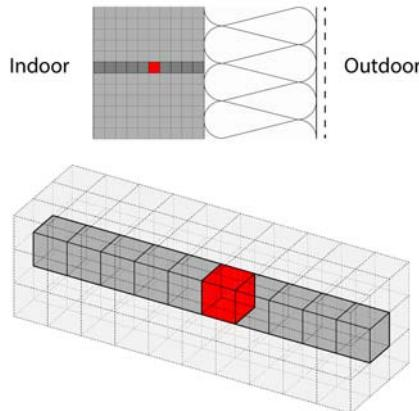
The setup used for the development of the envelope is as illustrated on Figure 3 consisting of three zones; an internal environment, an external environment and a wall section between the two. The external environment is defined by wind direction, wind
