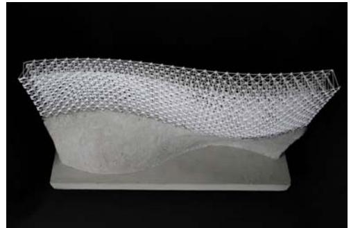
**Indirect intervention / reinforcement / formative and additive.** To overcome the complex and manual labour process of creating steel reinforcement cages, the "Tailorcrete" research project has explored the automation of this process through the formative process of robotic bending[4].
