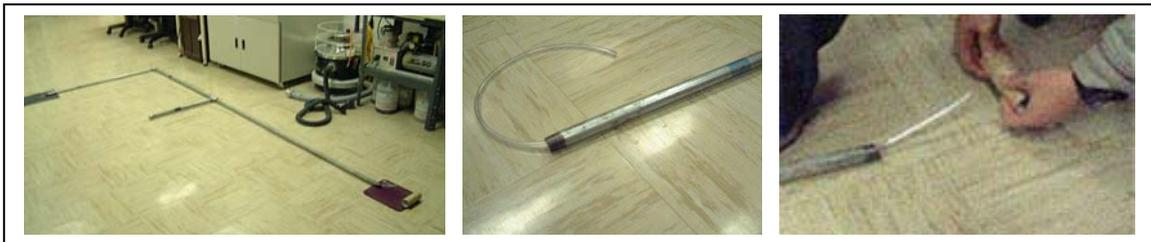
Fig. 3: An installation to test gas leakages (pressure drop) in the pipelines buried inside concrete
