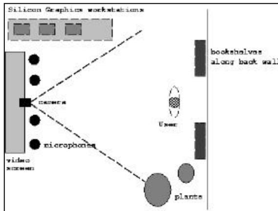
**Figure 3. Smart room setup including a single camera for body tracking, a microphone array for speaker identification, and a large projection screen for content viewing**
