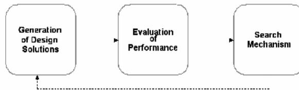
Figure 2 represents a diagram of the methods used in this paper for each of the GDS modules. In the search mechanism, Pareto Genetic Algorithms are used, which can handle multi-objective optimization problems without resorting to the use of arbitrary weighting factors and instead look for the best possible trade-offs between conflicting design objectives.
