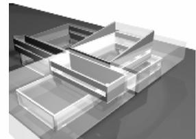
▲ Figure 7. Spaces being generated within the given rules and constraints. Translucent boxes represent upper bound constraints for each space, while opaque planes represent the spaces generated by the GDS
