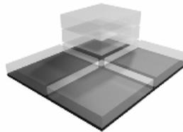
▲ Figure 5. Graphical representation of 2nd floor rooms maximum constraints. Space height can vary between 3 and 6 m. The topmost volume indicates maximum roof height
