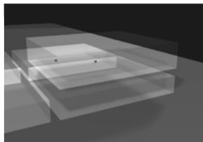
▲ Figure 6. The two dark dots represent daylighting sensors automatically placed by the GA inside a 2nd floor room
