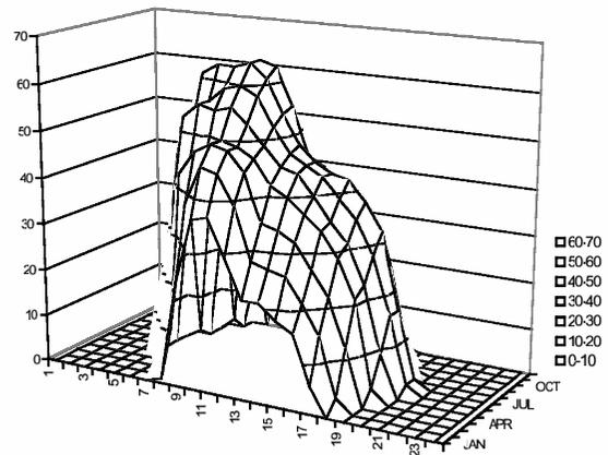
▲ Figure 15. Artificial lighting savings due to daylighting use, solution #1. Left: Room 3. Right: Room 7
