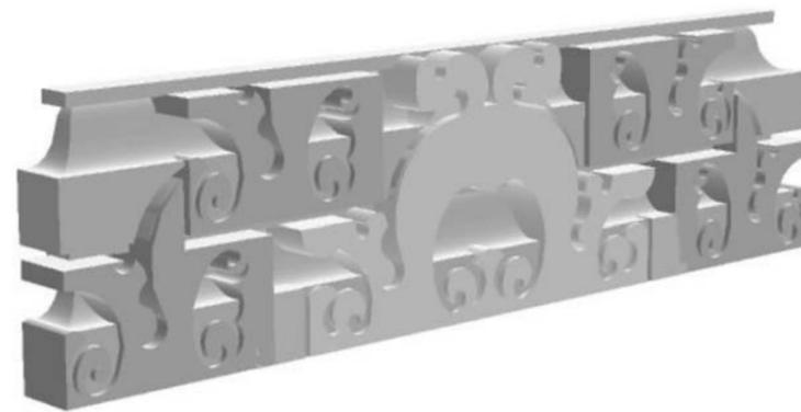
◀ Figure 6: The local geometry of the central spine is computed into a three dimensional tile made of a bounding box and two interlaced segments, a band model and units composed of carved pattern (gavaska patterns).
