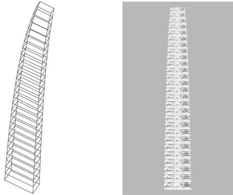
◀ Figure 7. Left: The skeletal geometry of the central spine is subdivided into constituent units based on a series progression. Right: A tiling function replaces each constituent unit in the series with self similar motif geometry.
