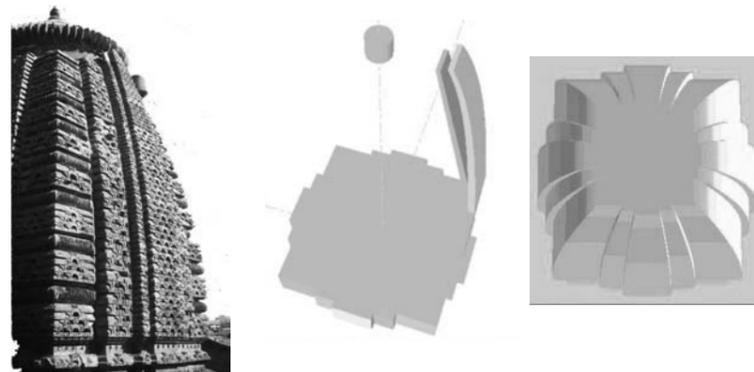
◀ Figure 2. Left: Surface Geometry of a temple with three offsets (four faces) showing the curvature. Middle: A generated example showing a base with three offsets, central axis and geometric envelopes of the central spine (offset). Right: Top view of a generated example showing the global model of the surface geometry.
