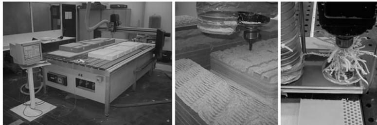
In most projects a 3-axis milling machine is used. For the fabrication of surfaces, and specifically of ornaments, the mill is appropriate as it is analogous to a “sculpting machine”. It is a simple, proven, inexpensive, and robust technology. The constraints of a 3-axis mill reside in the fact that it cannot do undercuts. This limitation is seen as a positive influence (especially in the teaching) as it forces additional reflection on the fabrication process while in the digital design stages.
