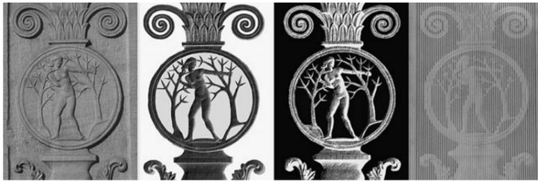
◀ Figure 5. An original image versus two image based manipulations and their milled output
