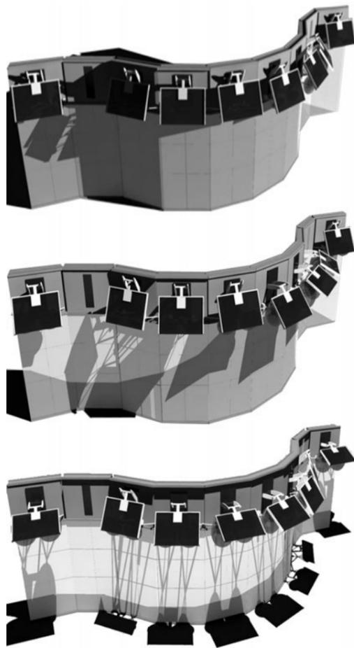
◀ Figure 5. Shade sequence for Heliotropic wall: in response to shifting solar conditions the photovoltaic shading petals protect the building envelope and form a shaded pedestrian pathway along the edge of the structure. Credit: Shane Ida Smith.
