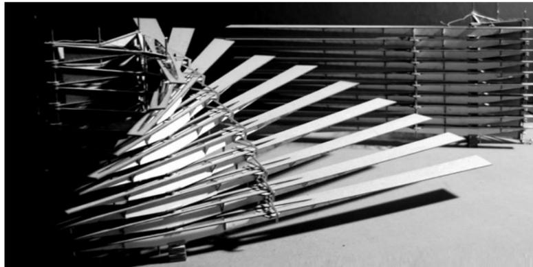
The final prototype is an array of ten cantilevered solar collection/shading blades. Activation begins at sunrise when the top photovoltaic blade collects solar radiation and triggers the coupled actuator. The first blade rotates laterally 10 degrees exposing 90% of the second
