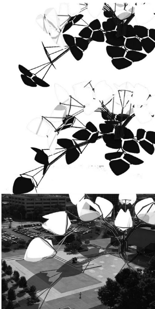
◀ Figure 4. Branching Heliotrope showing shade configurations: responsive to light for actuation, this trifurcating system allows multiple assemblies able to adjust to a variety of urban spaces generating a diversity shading patterns. Credit: Ryan Meeks.
