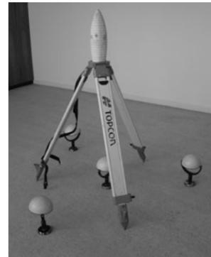
Set up for the 4 spherical targets and model
