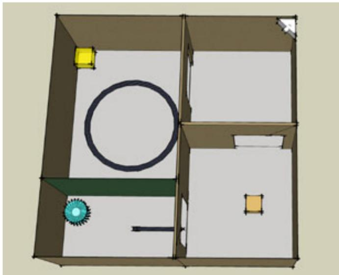
◀ Figure 3: Computer model of the augmented environment: a series of rooms with simple tasks, obstacles and sensory stimulations. The mobile sensor robot signals to the environment to raise the screen to enable it to complete a circuit.
