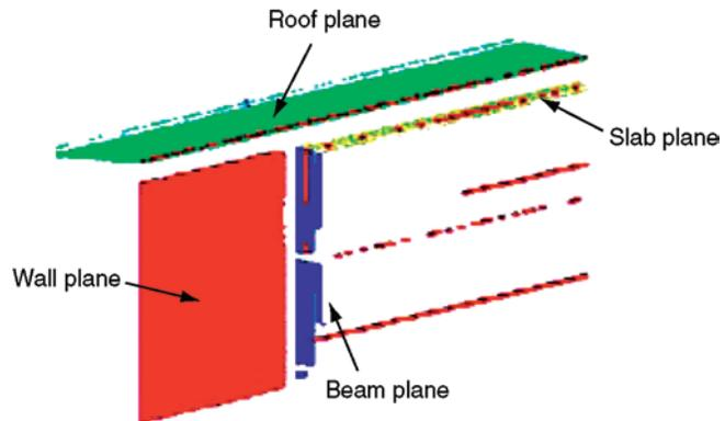
Figure 2. In this example, the plane depicting the wall plane (red one) was extracted firstly because it contains a large number of points. Consequently, it takes into account all points fulfilling within some threshold the flatness criterion, independently of any architectural constraint.
