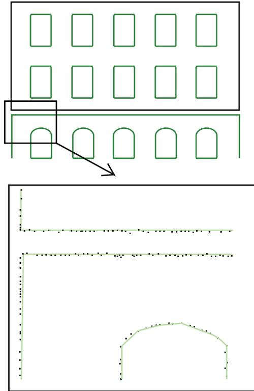
The manual digitizing is carried out by drawing straight lines and arcs in the raw point cloud. To quantify the quality of the position of contour points, distances of each point to the corresponding straight line are computed. The straight line is defined by its extremities (red points in Figure 22). Then the detection accuracy is defined as the standard deviation of distance values. In this study, the accuracy of straight contours extraction is  $\pm 2.5$  cm.
