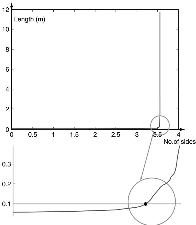
◀ Figure 10. Curve of lengths of triangle sides resulted from Delaunay triangulation and zoom on the point fixing the threshold (threshold value set at 0.1m here).
