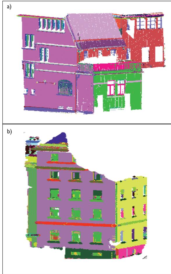
At this stage, the main new idea exploited in this algorithm is based on the hypothesis stipulating that contour points belong to the long sides of Delaunay triangles. Figure 9 shows that long sides are at the boundaries (wall contour and windows contours). The contour points are the extremities of the long sides. Therefore, lengths of all triangle sides are calculated and sorted in ascending order (Figure 10).
