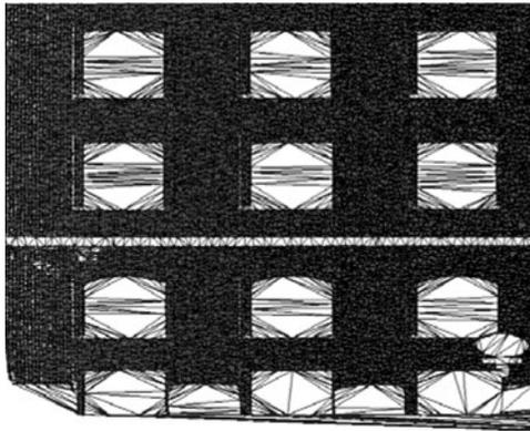
◀ Figure 9. Delaunay triangulation of a point cloud captured on a building façade.
