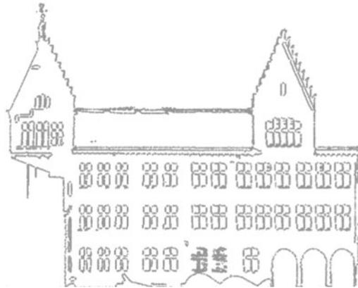
has also been tested on planes containing decorative architectural details (Figure 17). Despite the high level of details like ornaments, it gives satisfactory results (Figure 18). Therefore, if the quality of data and their segmentation is good, the algorithm can successfully be applied simultaneously on large and small details.
