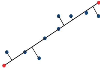
◀ Figure 22. Offsets between contour points and a straight line digitized manually.
