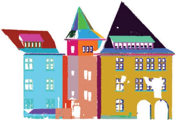
◀ Figure 19. Adjacent façades segmented into principal planar surfaces and features.
