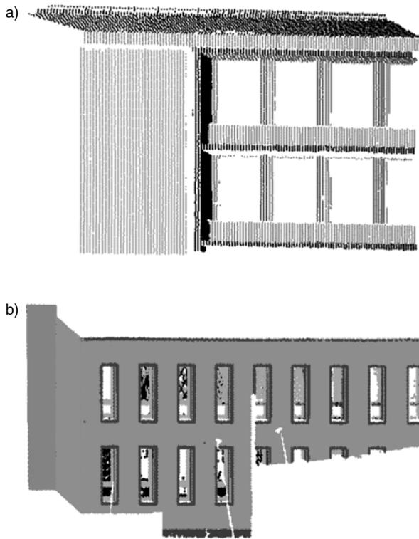
◀ Figure 7. Results of the application of the improved segmentation algorithm on simple building façades; a) small point cloud with low density; b) bigger point cloud with higher density.
