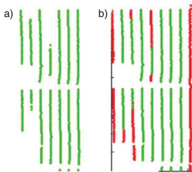
◀ Figure 5. Detection of points belonging to a plane; a) before correction; b) after correction (red points are retrieved).
