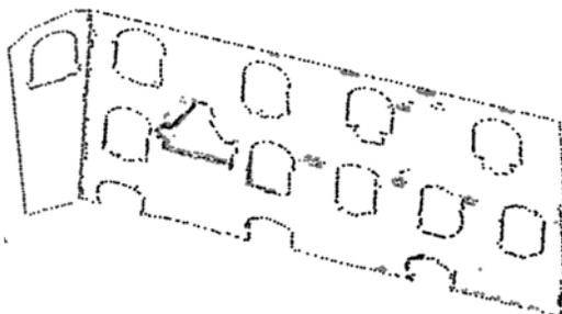
◀ Figure 16. Outer and inner contour points detected by the contours extraction algorithm.
