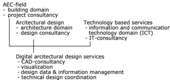
◀ Figure 2. Digital architectural design services combine IT-based services with building knowledge supplying design and construction.
