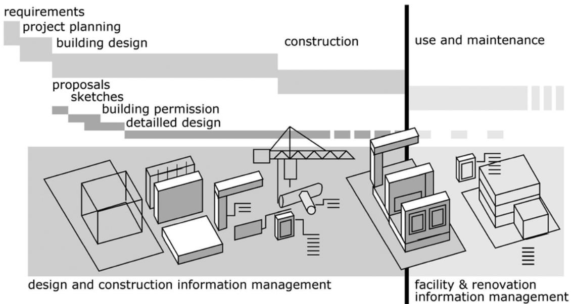
▲ Figure 3. The AEC-domain, building process phases before the building is completed, constitutes the scope for the services in this exercise. Facility management sector is excluded from the study.
