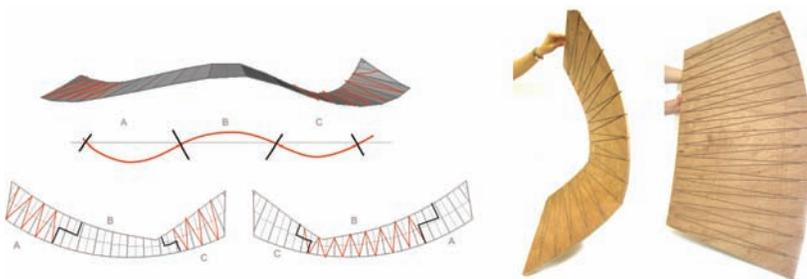
◀ Figure 4: Groove patterns and densities determined according to the desired bending (left), tests of the groove patterns and bending characteristics with plywood (right).
