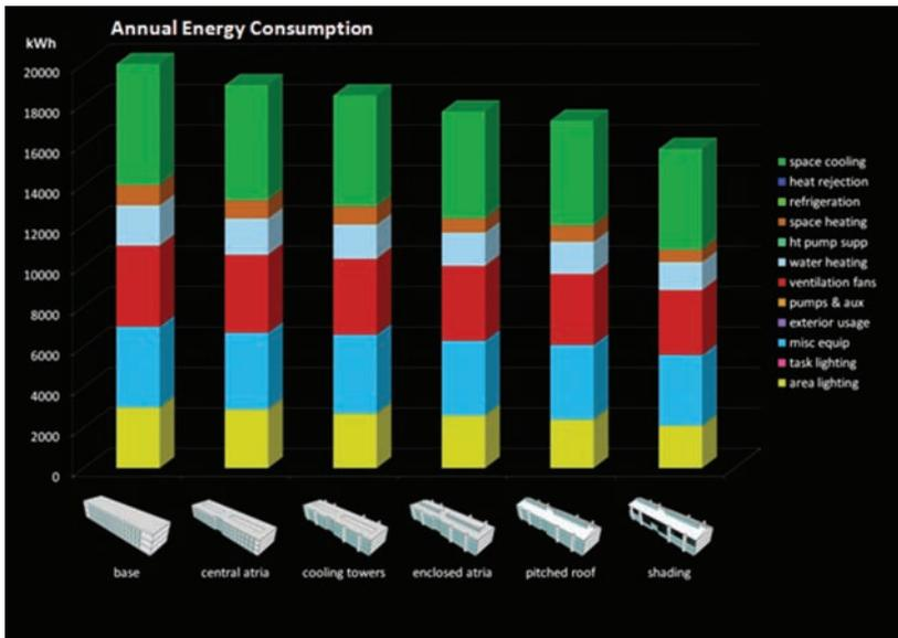
◀ Figure 9: Comparative visualization of energy simulation results
