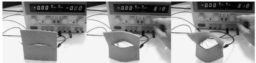
► Figure 22: Early stage of the experiment with individual modules of the 'eye-like' aperture actuated by SMA wire through DC electric power supply regulator.
