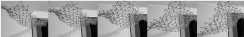
◀ Figure 4: Initial test of Elastic Space-Frame as skeleton that perform as contract and expendable skeleton.
