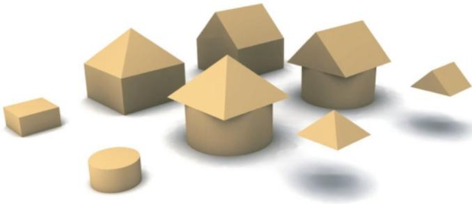
For our example therefore only four building blocks or, as we will call them from now on, *geometric primitives* are necessary: *cuboid*, *cylinder*, *prism* and *pyramid* (Fig. 3).
