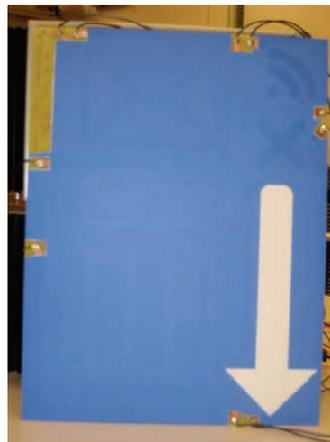
'draw' the patterns we wanted to eventually display on the thermochromic panels using CAD software, and then print these patterns in copper using one of several well-established techniques for producing PCB's from a CAD file.
