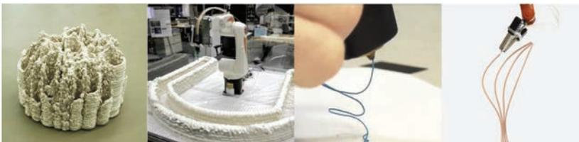
◀ Figure 6: Extrusions of polymeric material: The Foam [10], Building-Scale 3D Printing [11], 3Doodler [12], Mataerial [13]
