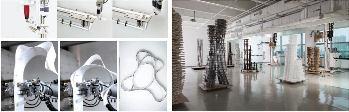
▲ Figure 2: Two selected fabrication concepts designed by the students: Top left: Bending setup. Acrylic stripes are fixed in a linear rail and pulled forward to their designated bending position. The material gets heated by a hot air gun to 550°C for 10 seconds. The robotic arm can now bend the material to any angle between 0° and approximately 160°. After the deformation the material gets cooled down by air pressure. Students: Kramer, Stünzi.
