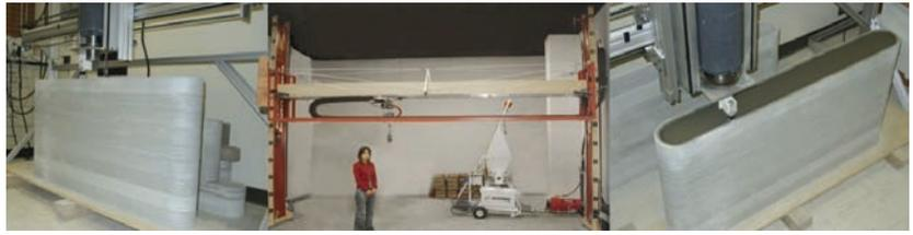
be used for the fabrication of geometrically unconstrained formwork and how through co-extruding of a tensile active filament this formwork could simultaneously act as reinforcement.
