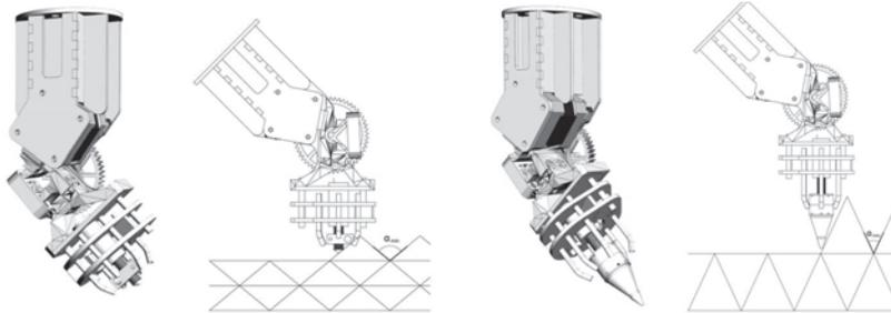
◀ Figure 12: Extruder head with air cooling: Based on standard components (left) and with custom extruder nozzle (right)
