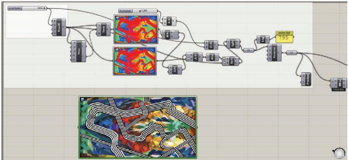
► Figure 4: Once the image was analyzed, the script produced the stained-glass pattern via a series of curves.
