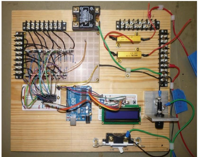
The electric current required to actuate the SMA wires far exceeded the maximum current output of an Arduino pin. For this reason, some type of transistor was needed to act as a switch for a higher-capacity power supply. The transistor used for the Pop-Op electronic control system was a Logic Level N-Channel MOSFET.
