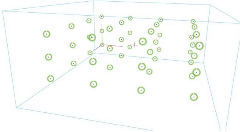
Figure 4 A right-angled and equally spaced speaker configuration to form an omnidirectional listening area.
