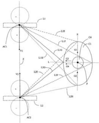
Figure 2 A phantom loudspeaker: two loudspeakers that are present at the same side of an ear are directed towards each other's acoustic centre make a non-localizable, virtual loudspeaker
