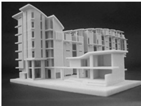
Fig 3. Model produced by rapid manufacture
