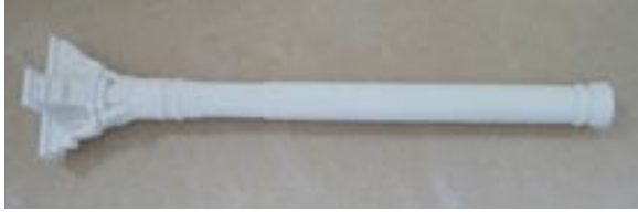
Figure 5: Example of detailed column created by means of 3D-printing.
