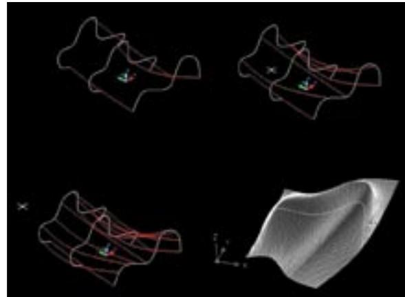
Figure 1: Spline subdivision script to create an approximate spline surface in autocad.
