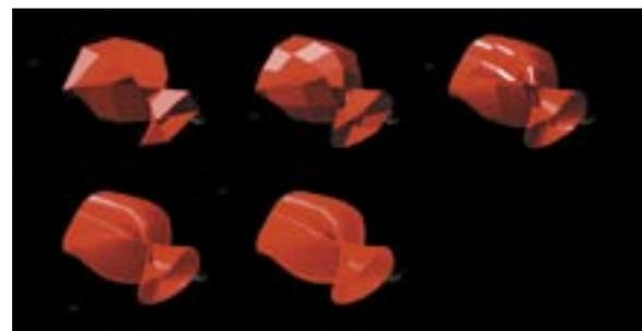
Figure 2: A subdivision factor is set as a variable, adjusting the smoothness of the resulting approximated spline surface.
