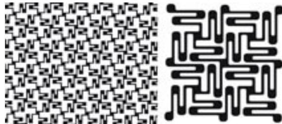
Figure 5: Flexure pattern propagation and final pattern developed, with rounded edges avoiding fracture points
