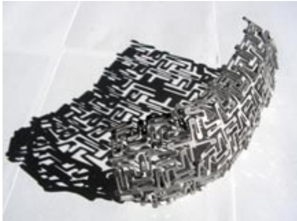
Figure 7: Double curved structure fabricated from a rigid flat aluminum panel
