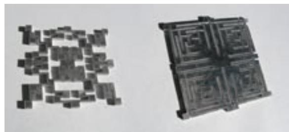
Figure 6: Flexures fabricated with a CNC Water Jet machine on 4mm aluminum
