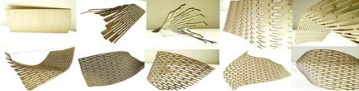
Figure 3: Different results obtained from processing equal panels with the same script but with different variable values
