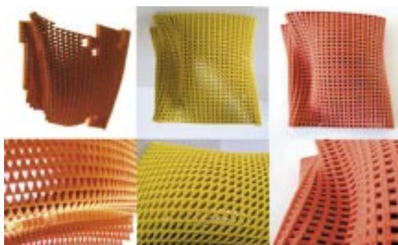
Figure 8: Double curved structures developed through solid module scripting and 3D printed using a ZCorp Machine
