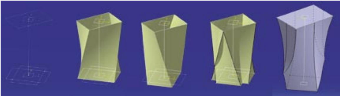
Figure 3: Rectangular knot generated from the same parametric model. The square is transformed into a rectangular shape and the angles and the column height are changed accordingly.
