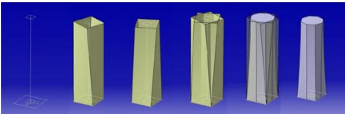
Figure 2: Generation process of the column. Parametric skeleton, surface fitting for rotation and counter-rotation and Boolean intersection.
