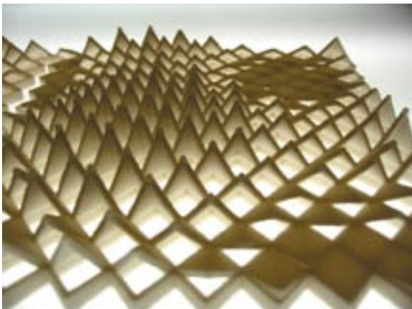
Figure 6: Surface effect pattern printed on ZCorp to test light/shadow performance.
