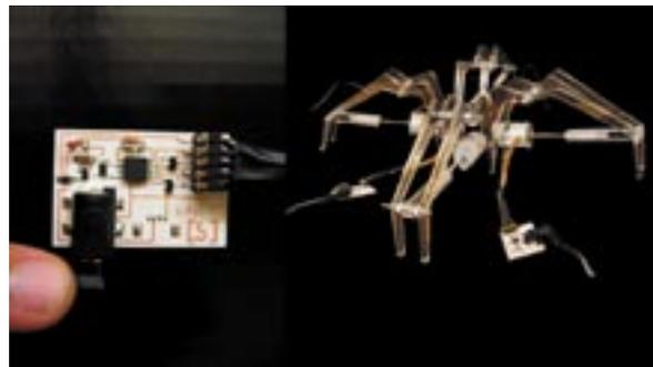
Figure 8: Microcontroller and actuator node using four solenoids created from stepper motors.
