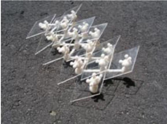
Figure 2: Articulated spider prong joints provide independent operability for each scale feature
