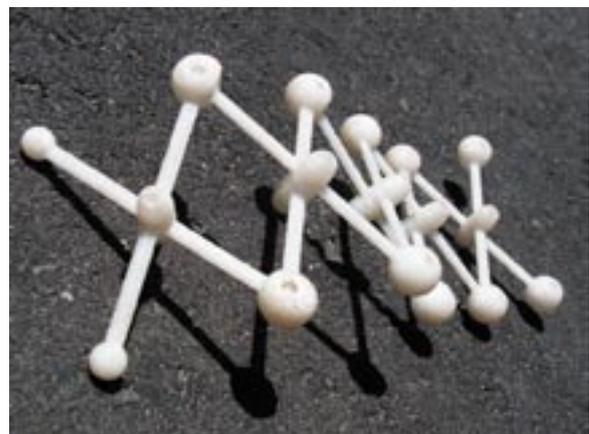
Figure 1: The spherical articulation provides double curved deformation on diagrid structure.
