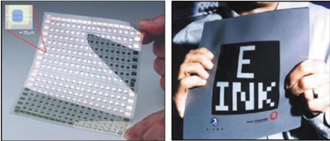
Figure 3 Flexible electronic circuit (left) and paperlike display system constructed with it (right).
