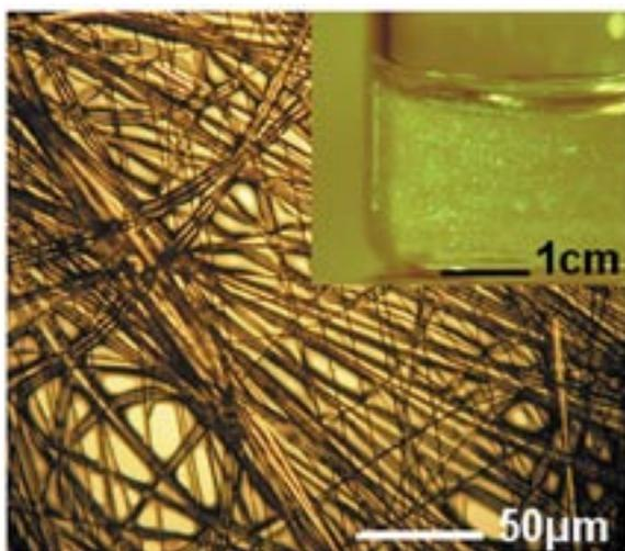
Figure 4. Microstructured silicon, in the form of long narrow ribbons. The inset shows a solution suspension of this material.
