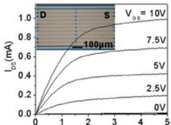
Figure 5. Current-voltage characteristics of a device that uses  $\mu\text{-Si}$  as the semiconductor.
