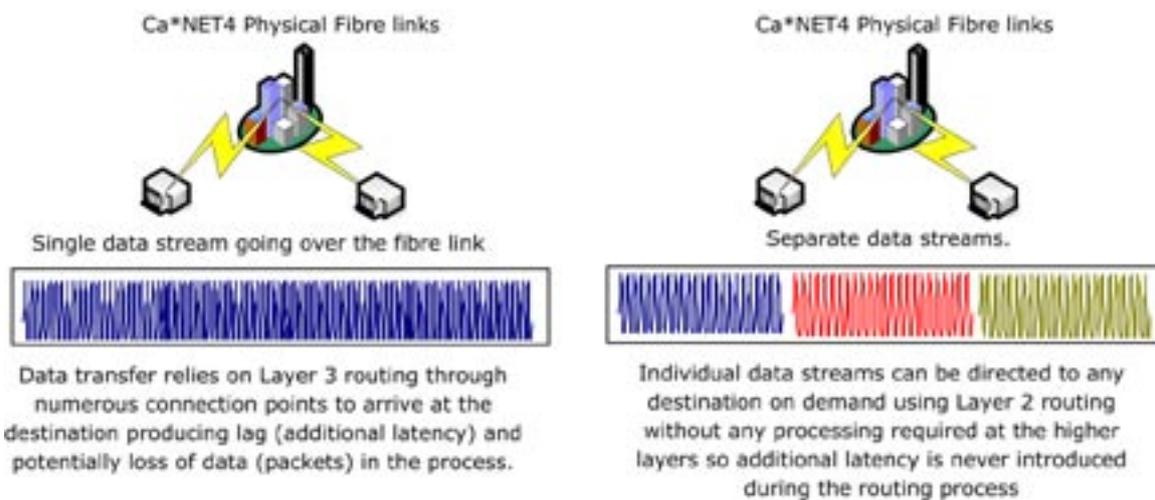
Comparison of a single and multiple streams utilizing WDM.
