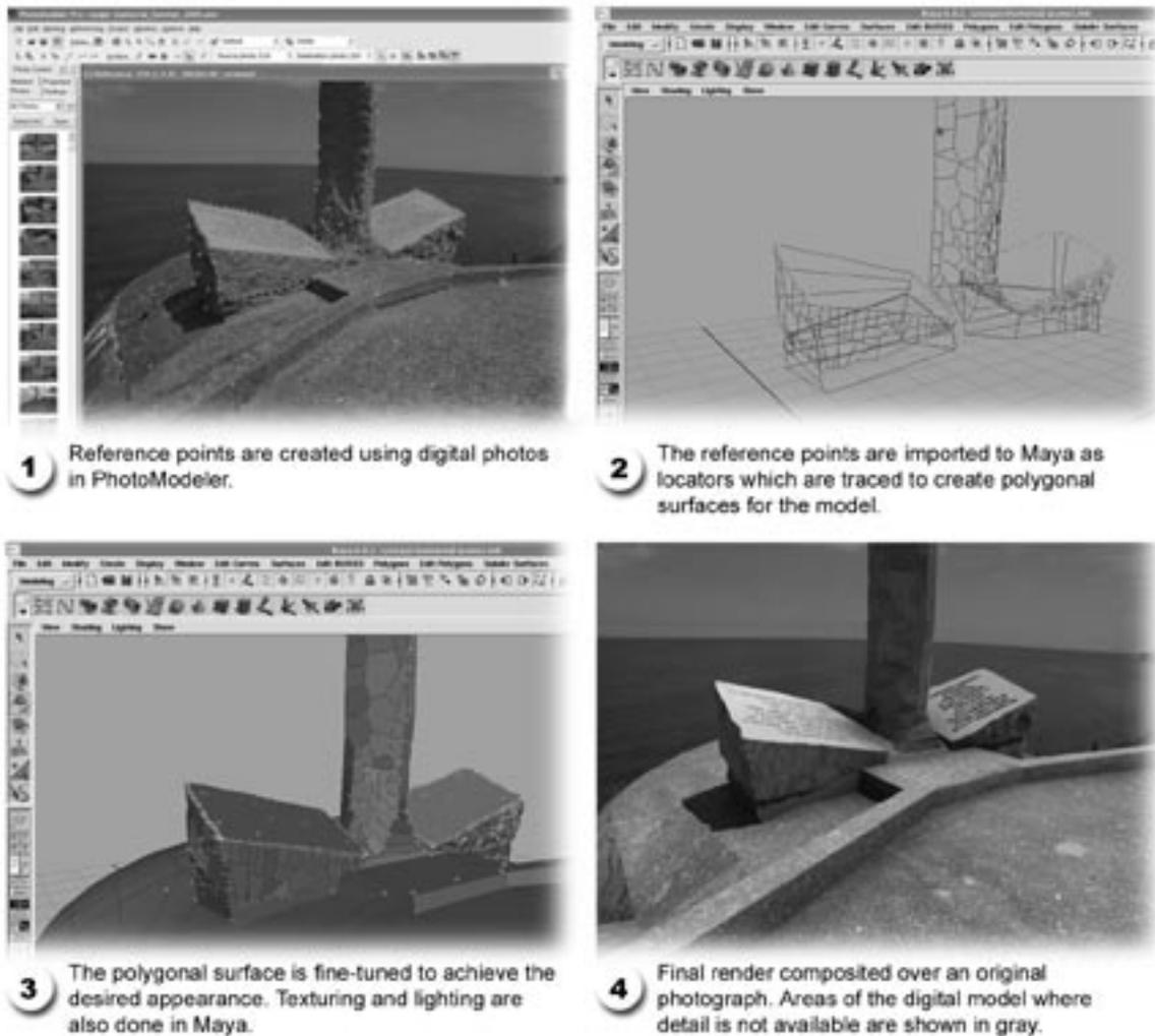
Figure 2: Digital reconstruction process.
