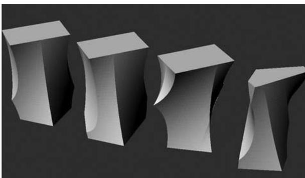
Figure 2. Parametric Model for Exploratory Design. Different design configurations are produced with a single parametric model.
