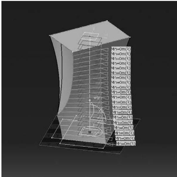
Figure 4. A parametric model that shows the properties of the surface curvature. The information on the curvature will be updated every time the design is changed allowing the designer immediate access to this information.
