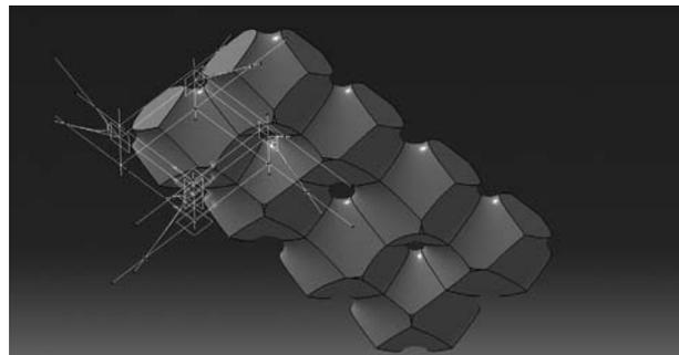
Figure 3. Reusability of a parametric model. One parametric model is used in different scenarios through duplication and local adaptability.
