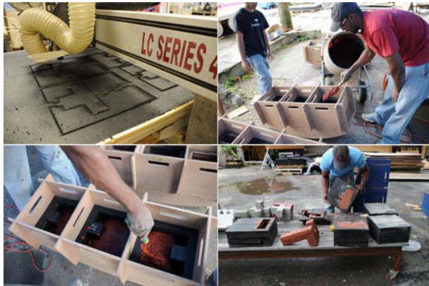
Fig. 7. Physical prototyping of CNC-cut layered mold system and casting of components.
