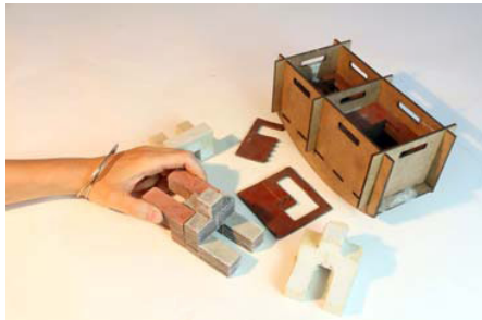
Fig. 6. A prototype laser-cut mold-making device with cast components.
