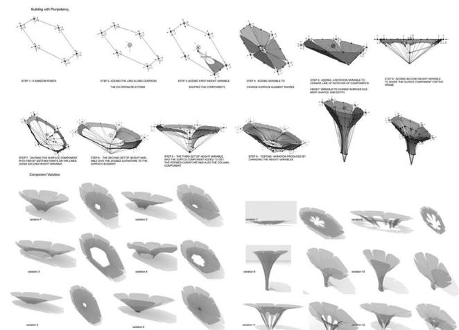
Fig. 2. The design of the pluripotent components, which is aggregated over the base surface. The above fig shows the various kinds of profile and form the base pluripotent module can take simulating the concept of pluripotency.
