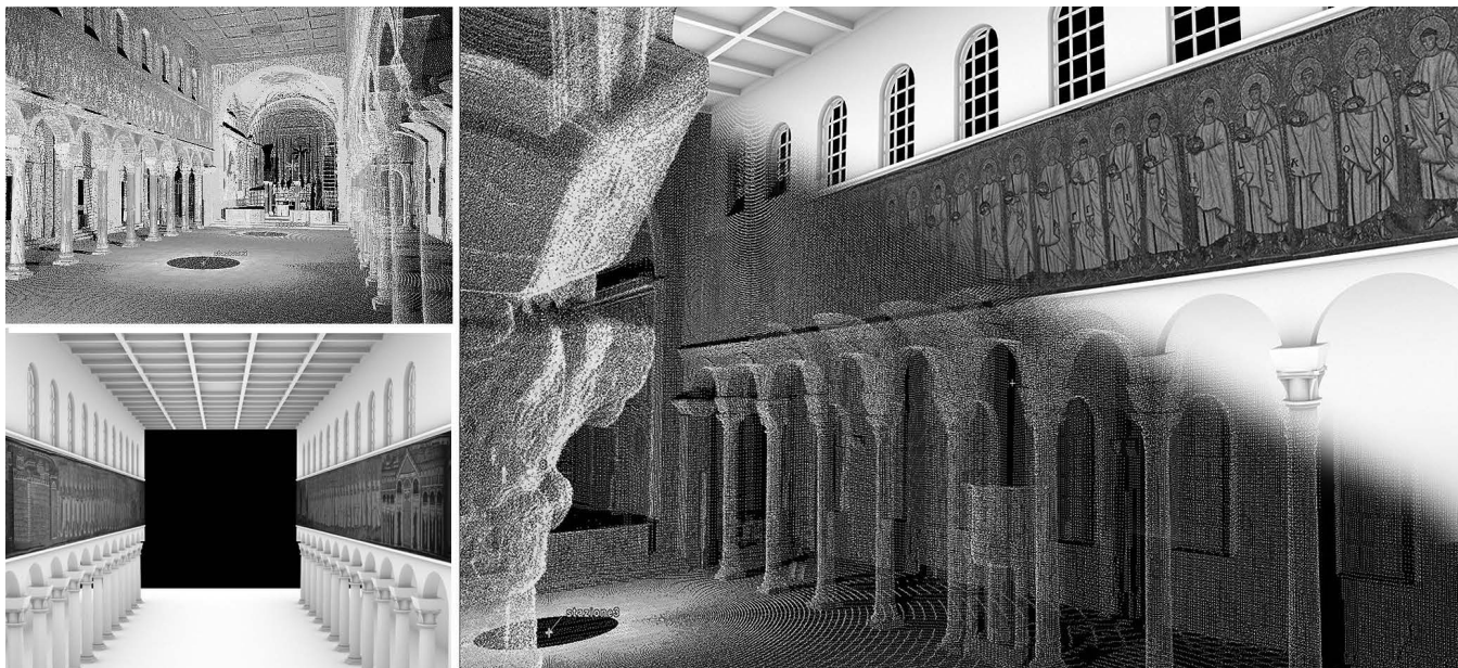
Fig. 3. Once a 3d model has been generated with BIM software, visual analysis is easier: this is the final registration of several point clouds representing Sant'Apollinare interiors, with important mosaics on walls.
