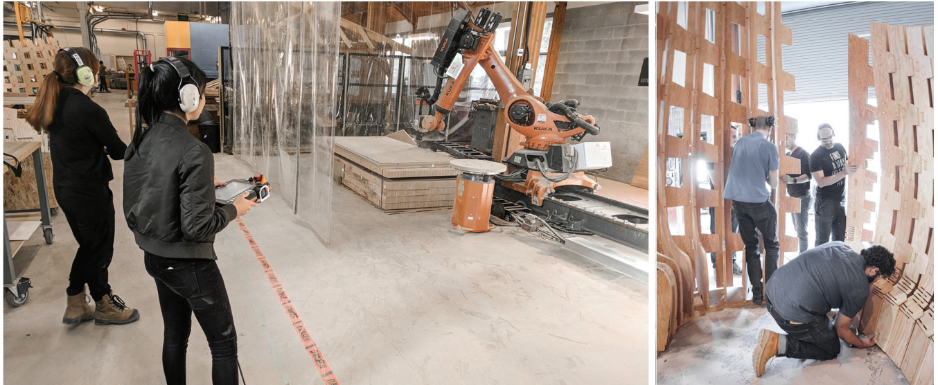
5 Robotic fabrication and modular assembly process: Each piece was cut in a 5-axis CNC process using an extended 7-axis robotic setup; thereafter, the elements were assembled in the workshop under controlled conditions into 5 separate modules small enough to be transported across campus, and the modules were then assembled on site into the final demonstrator
