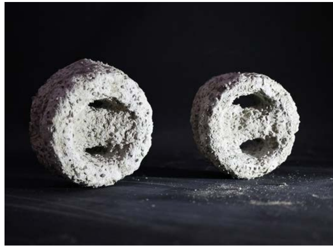
12 Uniform mixing ratio composite and a layer thickness of 5mm. Left: 2mm binder spacing (continuous pattern); Right: 3.5mm spacing (image monitoring to fill gaps).
