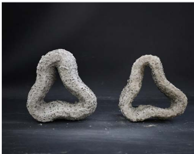
13 Different mixing ratios on layer thickness vary from 3mm, 5mm, and 8mm. Left: 2mm binder spacing (continuous pattern); Right: 3.5mm spacing (image monitoring to fill gaps).
