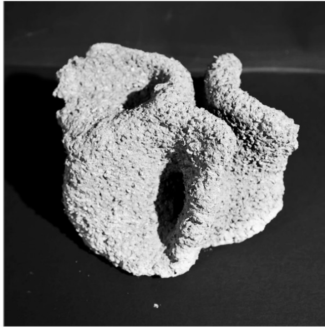
16 Final Print Product; as demonstrated by the juxtaposition of the digital model and its physical counterpart, substantiates our system's adaptability to different mixing ratios and layer thicknesses, delivering commendable shape accuracy. This showcases our system's proficiency in managing diverse printing tasks, upholding precision and quality across various conditions.
