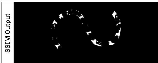
9 Leveraging the Structural Similarity Index Measure (SSIM), we identified discrepancies between the actual printed pattern and the original digital model. This analysis helped pinpoint the contours of missing parts, thereby enabling precise corrective binder placement in the subsequent stages of the printing process.
