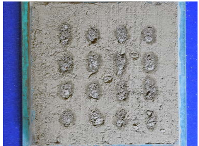
7 Shortline printing test (Cement: Sand: Aggregate = 1:1:2).
