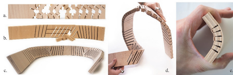
Figure 2.a. Failed sections during the machining process. b. The section failed due to inappropriate geometry and order of cuts. c, d. Similar section after editing the cut order and geometry. e. Delamination of the section
