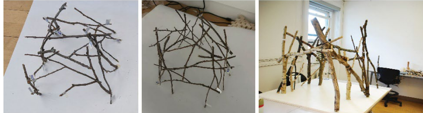
Figure 8. Fabricated structures built with augmented reality (AR) from irregular Y-branches. Structure A (left), structure B (middle) and structure C (right)
