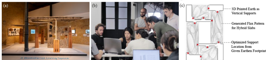
Figure 1. (a) Living Prototypes Exhibition, 2022, © Erik-Jan Ouwerkerk; (b) Hybrid material system design workshop; (c) Hybrid slab design outcome of digital tool, adapted from design workshop, 2022, © IAAC
